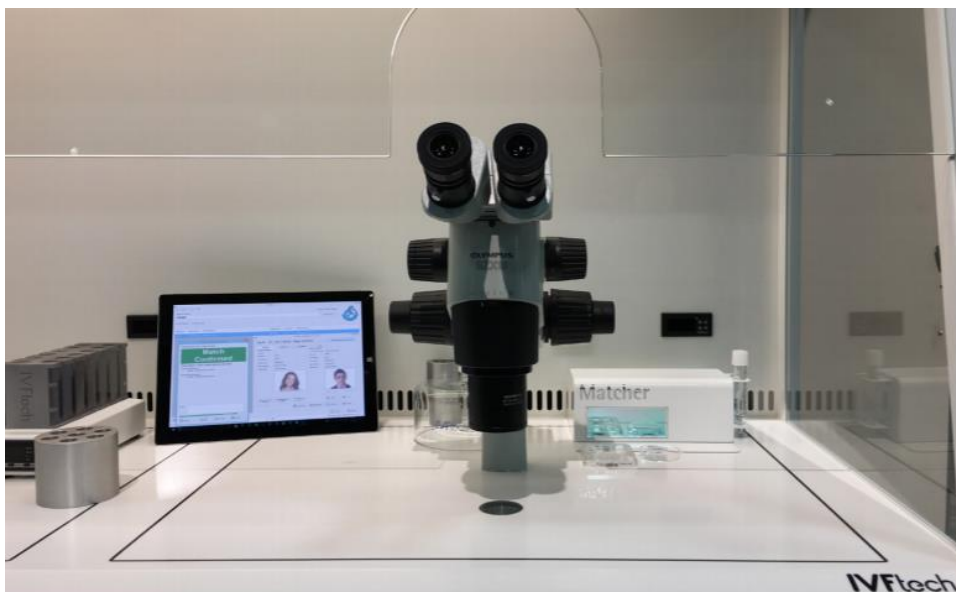
Typical installation in a laminar flow hood; the Matcher software is controlled on a touchscreen tablet and a Benchtop Matcher reads barcodes using inbuilt digital cameras.
