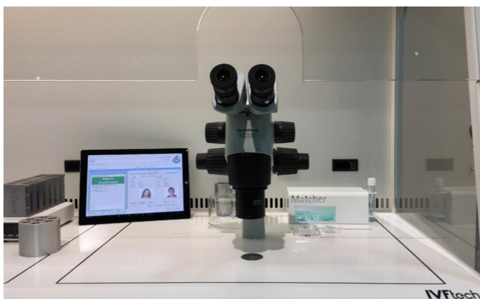
Typical installation in a laminar flow hood; the Matcher software is controlled on a touchscreen tablet and a Benchtop Matcher reads barcodes using inbuilt digital cameras.
